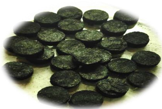
Figure 1 – Rice straw: oil sludge: activated carbon which was taken in the ratio of lignosulfonate 9: 1: 2
