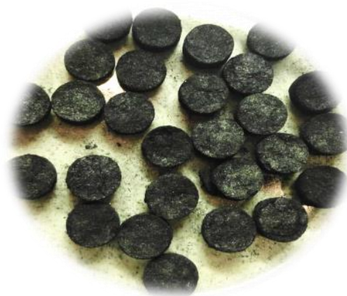
Figure 1 – Rice husk oil sludge: activated carbon obtained in the ratio of lignosulfonate 9: 1: 2.
